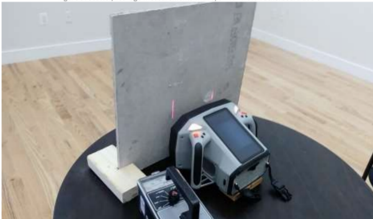
Figure 9: Scatter/Leakage Measurements with 3/8" Concrete Backerboard at 5 c
