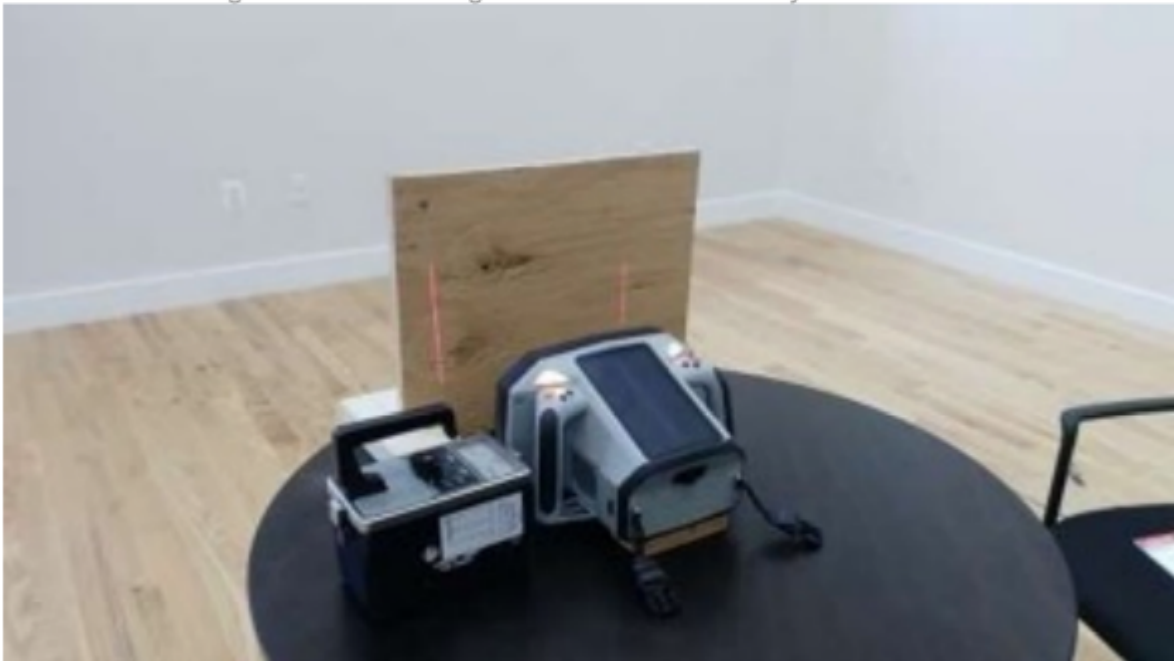
Figure 8: Scatter/Leakage Measurements with \frac{3}{4} " Plywood at 10 cm
