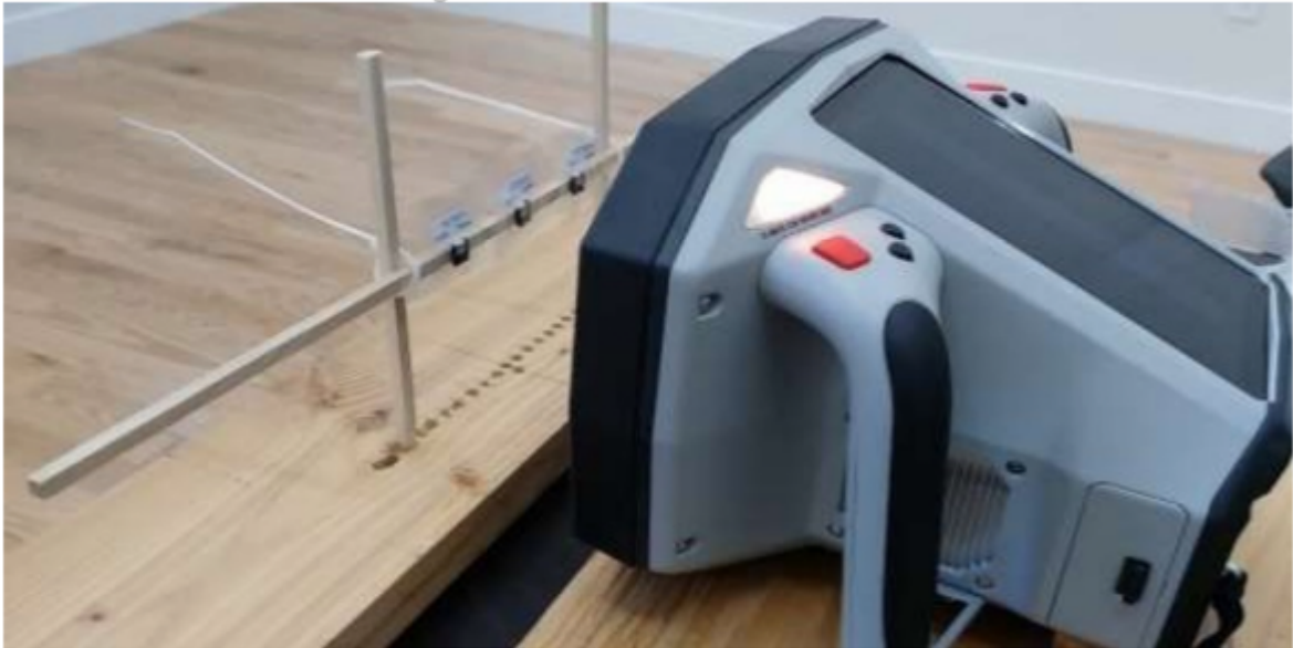
Figure 8: Scatter/Leakage Measurements with \frac{3}{4} " Plywood at 10 cm
